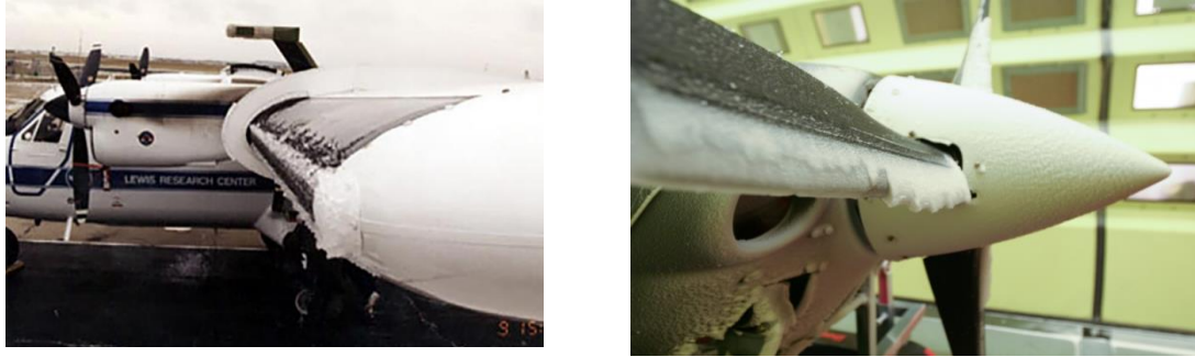
FIG. 1.1 Ice buildup on aircraft surfaces, [2, 3]
